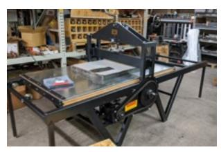
Custom built by Takach in Albuquerque, NM, the new press has a bed size of 40" x 72", which increases the overall size of print that can be produced at CSIA. It features an electrically-driven motor with updated technology and locking mechanisms to accommodate both litho plates and stones. The press will be used as the primary publishing press for the studio, replacing the previous 30" x 64" 1977 Takach-Garfield brand press that had been the workhorse of the studio for the past 20 years.
